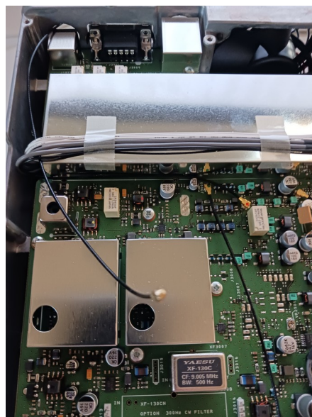
Figure.3 : U.FL to SMA cable installation.
