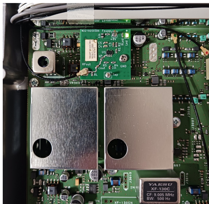
Figure.8 : Ready to use FTRX-10 panadapter installation.
